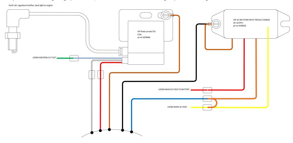
MB way... to bring the Vape AC with DC trickle charge inline with normal Lambretta colour coding - wire direct with connectors don't bother using the spares and extra wiring that comes in the kit
