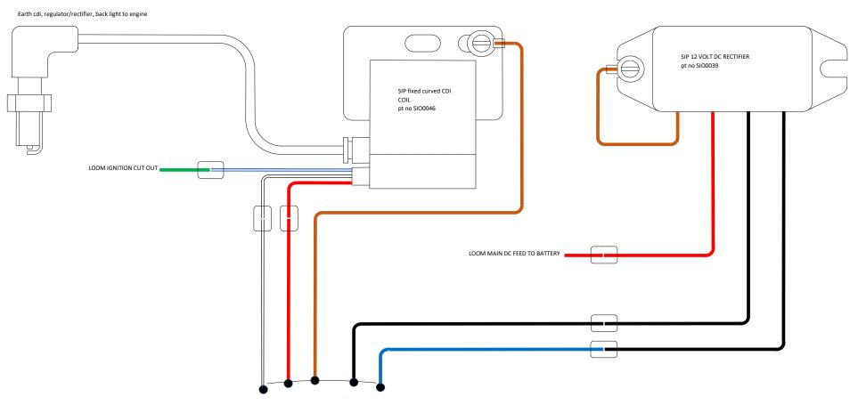
MB way... to bring the Vape DC inline with normal Lambretta colour coding - wire direct with connectors, don't bother using the spares and extra wiring that comes in the kit
