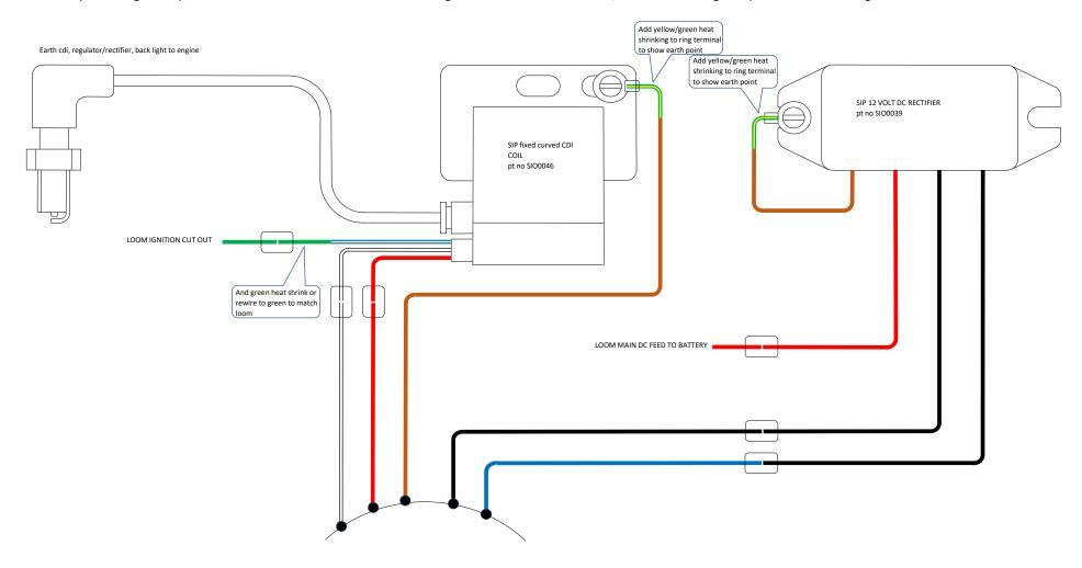
Vape AC with DC trickle charge wiring as per instructions, wire direct with connectors don't bother using the spares and extra wiring that comes in the kit
